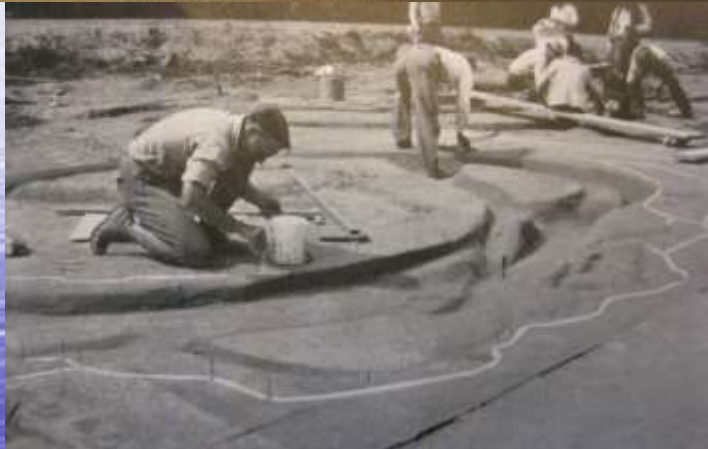
Model of Birds Point-New Madrid floodway under test
