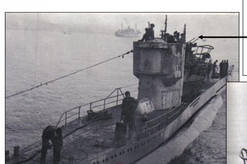
U-Boats were initially fitted with a single 20 mm AA gun; later increasing to two (shown at left) and then four barrel configuration, shown below
