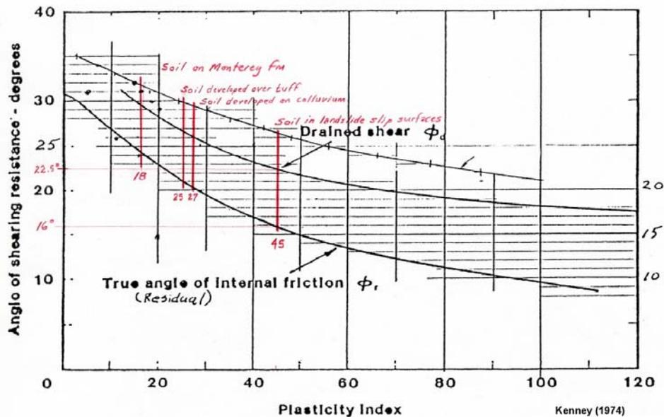
**Figure 4** – Plasticity data for residual soils and landslides developed on the Rincon Shale plotted in red on a chart comparing PI with residual angle of internal friction,  $\phi_r$ , taken from Kenney (1967).  $\phi_r = 16$  degrees appears representative of the largest bedrock slump-flow landslides developed in the weathered Rincon Shale.
