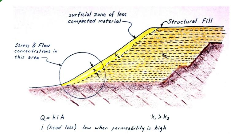
The low density zone along the face of a fill slope can be mitigated by: 1) trimming; 2) embedment of geotextiles, or 3) by emplacement of deep-rooting woody vegetation
