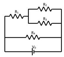
**13.** For the circuit shown: if the battery provides a voltage of 24 V, the current through resistor  $R_4$  equals \_\_\_\_\_\_ and the power dissipated in resistor  $R_4$  equals \_\_\_\_\_\_ A) 10A, 360W B) 4A, 96 W C) 10A, 600W D) 4
