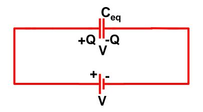
"equivalent" means it has the same charge Q and the same voltage drop V as the three capacitors
