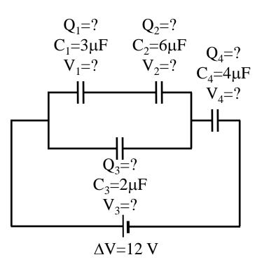
**Homework Hint**: each capacitor has associated with it a Q, C, and V. If you don't know what to do next, near each capacitor, write down Q = , C = , and V = . Next to the = sign record the known value or a "?" if you don't know the value. As soon as you know any two of Q, C, and V, you can determine the third. This technique often provides visual clues about what to do next.
