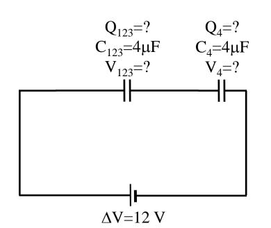
$C_4$  is in series with  $C_{123}$  and together they form  $C_{eq}$ .
