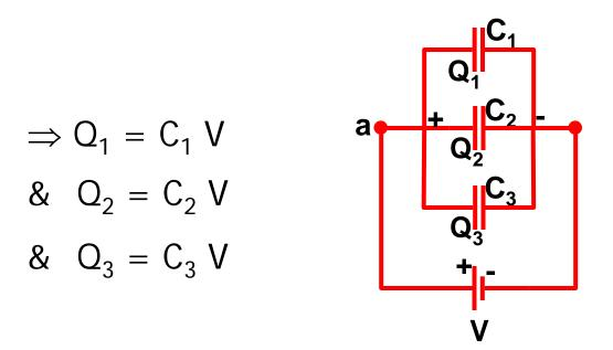
Imagine replacing the parallel combination of capacitors by a single **equivalent capacitor**
