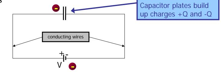
• when battery is disconnected, charge remains on plates
