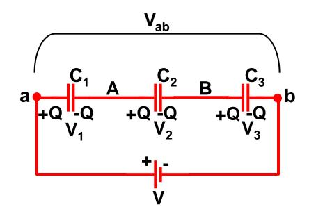
The charges on  $C_1$ ,  $C_2$ , and  $C_3$  are the same, and are  $Q = C_1 V_1$   $Q = C_2 V_2$   $Q = C_3 V_3$
