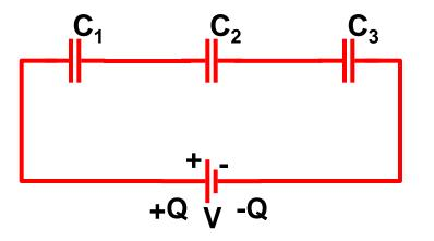
charge +Q flows from the battery to the left plate of  $C_1$
