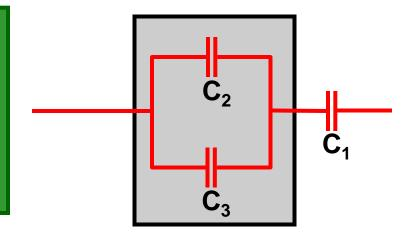
Start by combining parallel combination of C<sub>2</sub> and C<sub>3</sub>
