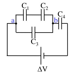
In the figure on this slide, if  $V_{ab} = 100 \text{ V}$  then point a is at a potential 100 volts higher than point b, and  $V_{a \rightarrow b} = -100 \text{ V}$ ; there is a 100 volt drop on going from a to b.
