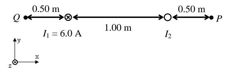
Two long parallel conductors are separated by 1.0 m. The wire on the left carries a current  $I_1 = 6.0$  A into the page. (c) If a third long wire is placed at P and carries a current  $I_3 = 2.0$  A in the –y direction, what is the magnitude and direction of the net magnetic field at point Q?
