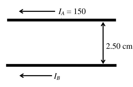
The magnetic force on wire B due to the current in wire A is
