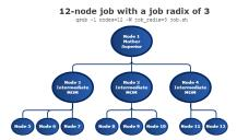
The Mother Superior picks three sister nodes with which to communicate the job information. Each of those nodes (intermediate MOMs) receives a list of all sister nodes that will be subordinate to it. They each contact up to three nodes and pass the job information on to those nodes. This pattern continues until the bottom level is reached. All communication is now passed across this new hierarchy. The stdout and stderr data is aggregated and sent up the tree until it
